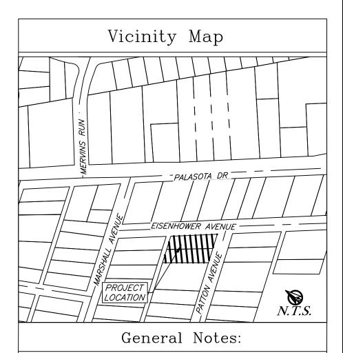
1. Bearing system shown hereon is based on the Texas State plane central zone grid North as established from GPS observation using the Leica Smartnet NAD83 (NA2011) Epoch 2010 multi-year cors solution 2 (MYCS2).
